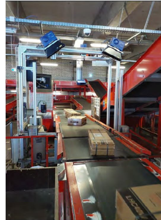
Singulated parcel-flow with conventional volume measurement system
