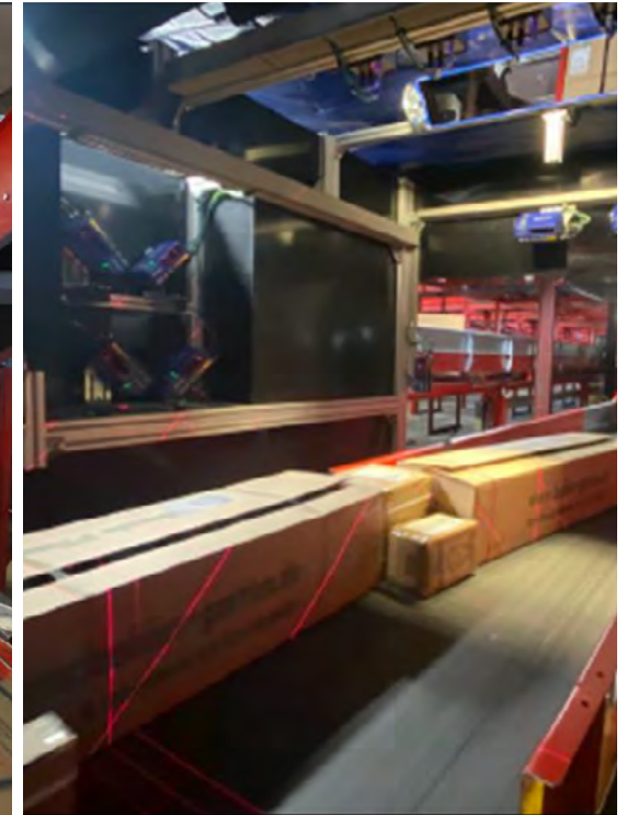
Parcels are conveyed in bulk, touching or side-by-side, while being identified and measured by the Mass-Flow-Detection-System
